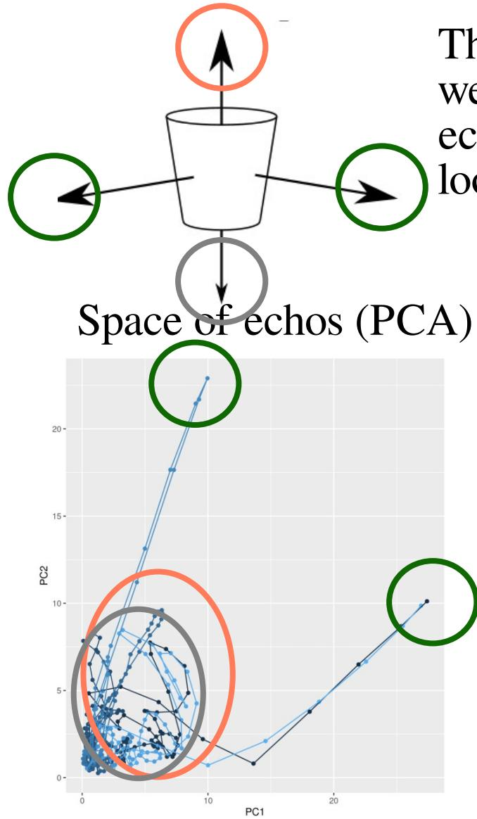
The top and bottom have weaker, wider beamwidth echos  $\rightarrow$  wider, smaller loops
